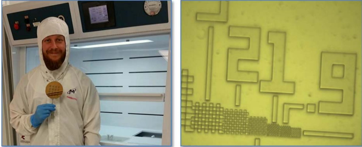
Figure 34. Graduate student Torrey McLoughlin (left) in MSU's Microfabrication Lab, holding chrome on silicon wafer that was coated with gold and photoresist and then exposed and developed to reveal 3, 2, 1.5, 1, and 0.9 micron features (right). The optimal exposure time was determined to be 1.4 second.
