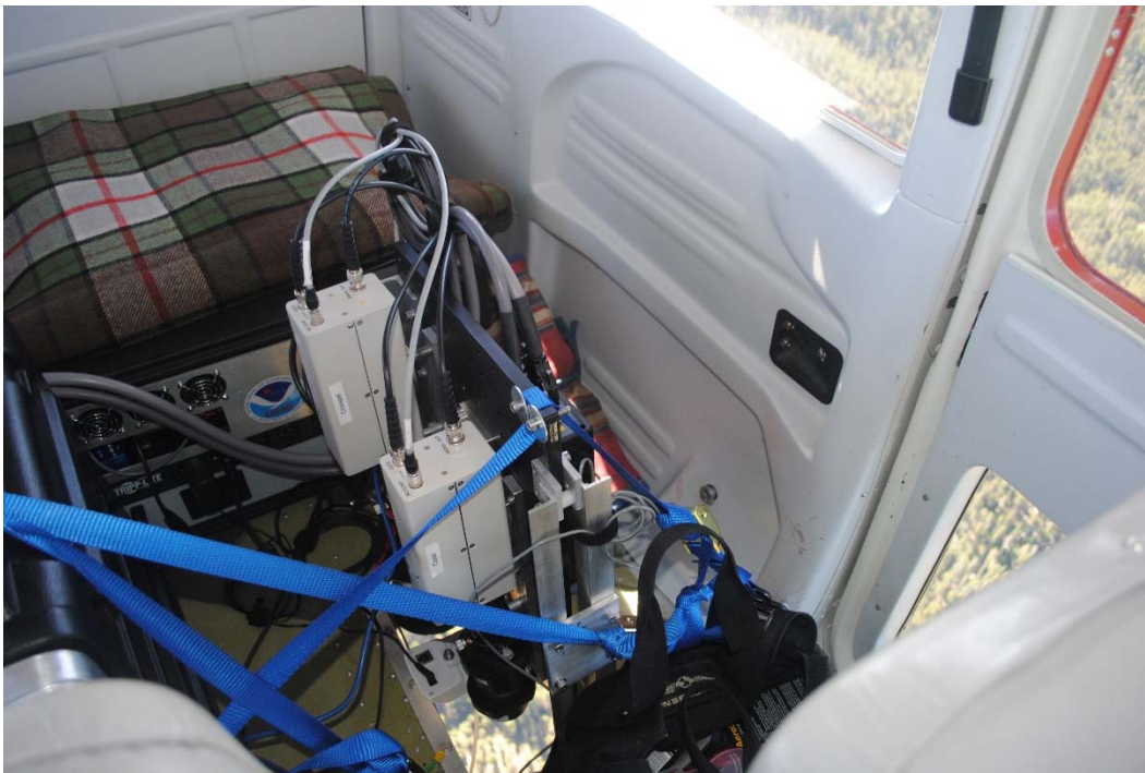
Figure 9. Photograph of the MSU airborne lidar installed in the rear of a Cessna 185. The two receiver telescopes and the laser are mounted above a hole in the cabin floor. The electronics, battery, and inverter sit behind the pilot and the lidar operator in the rear of the plane.
