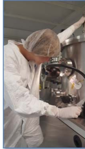
Figure 25. AdvR professionals working on waveguide fabrication processes with MSU personnel. (left) Briana Jones of AdvR prepares poled waveguide wafer for HF etch bath under AdvR's vented fume hood. (right) Sarah Mondl of AdvR positions a LN wafer in MSU's MMF Cobleigh Hall cleanroom within the Angstrom sputter system in preparation for SiO 2 deposition.
