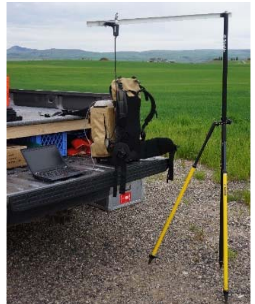
Figure 14. ASD spectrometer used to measure on-ground reflectance.
