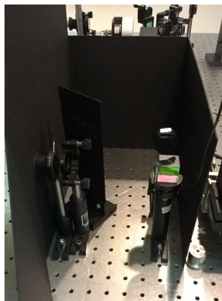
Figure 46. Outside and inside of the black box used for shielding the detector from the pump beam.
